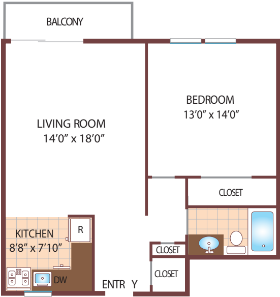
One Bedroom Efficiency Floor Plan Ground Floor Unit with 1 Bath, 725 sq. ft.
